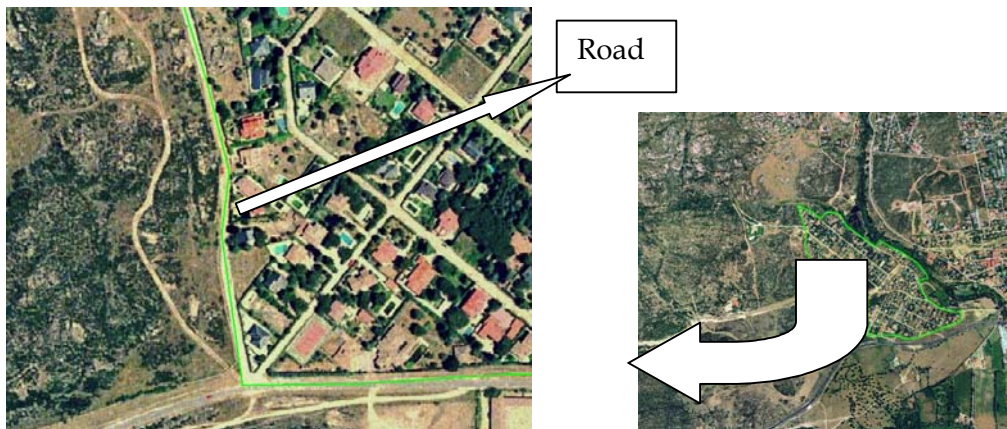
Fig1.- . Settlement with lots in the perimeter which are not considered in contact to forest fuel because they are surrounded by a road.
